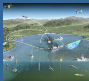
The MUSE project involved three ships, two aircraft, two satellites, two AUVs, several drifters, nine moorings, six gliders, and a host of small boats, designed to examine a natural iron fertilization event.
